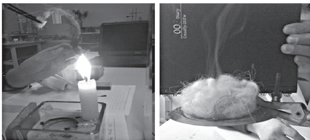
Picture 2. Burning process of fireproofed hair fibers
